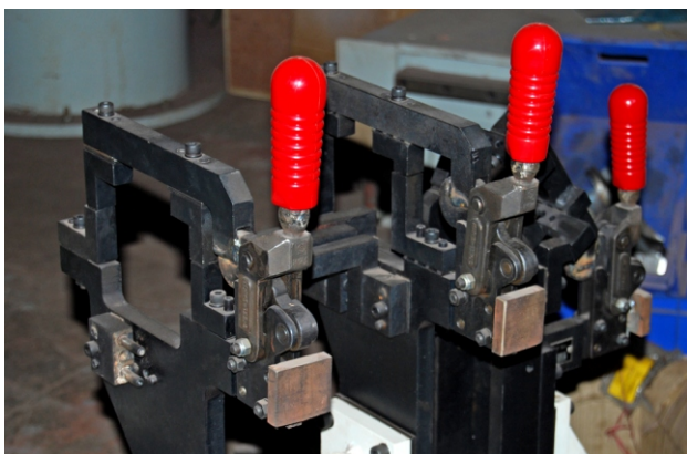
HV Series Clamp in a BIW fixture
