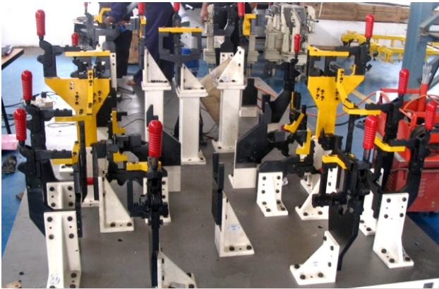
Numerous HV Series used in a Spot welding fixture
