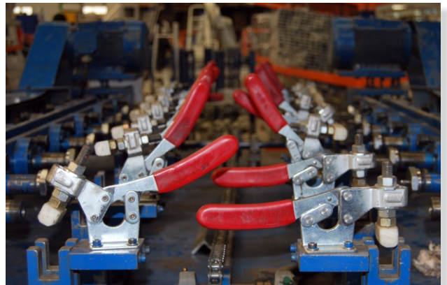
H - Series Clamps used for Ladder Assembly
