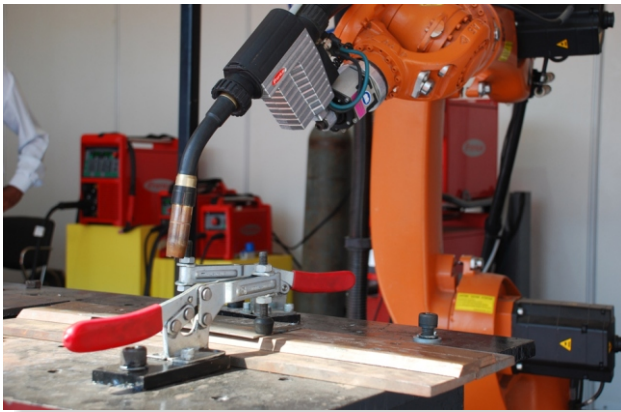
H-45105-UB on Co2 Welding fixture
