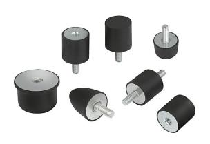
Rubber-metal buffers, type A Material & Version: Metal parts steel grade 5.6 or SS, Galvanized or bright. Elastomer natural rubber, Medium hardness, 55 Shore A.
