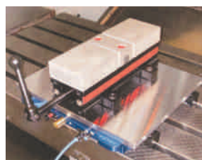
Example of standard pallet machined into a fixture plate positioned on base unit for increased production.
