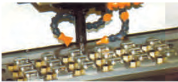
Cam action side clamping
