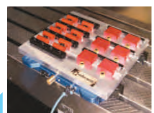
Example of standard pallet machined into a fixture plate positioned on base unit for increased production.
